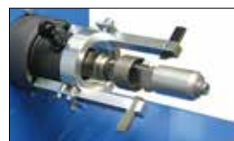
Simultaneous internal and external skiving.
