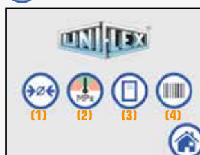
Four choices for selecting compression parameters quickly and easily. Selection menu includes pressing by dimension, by pressure, stored parameters in integrated database in the controller; or by use of a barcode scanner.
