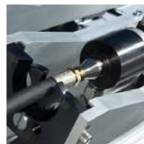
2 clamping discs per head, catering to various diameters (OD 8-42 mm).
